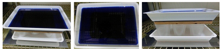
Fig.2 Appearance during nail water seal test
