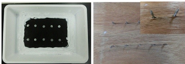
Fig.3 3040BK's appearance after 70days storage at 194F (20 equivalent year)
