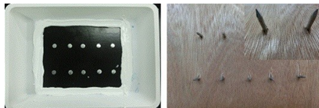
Fig.4 3040BK's appearance after 12days super UV exposure (20 equivalent year)
