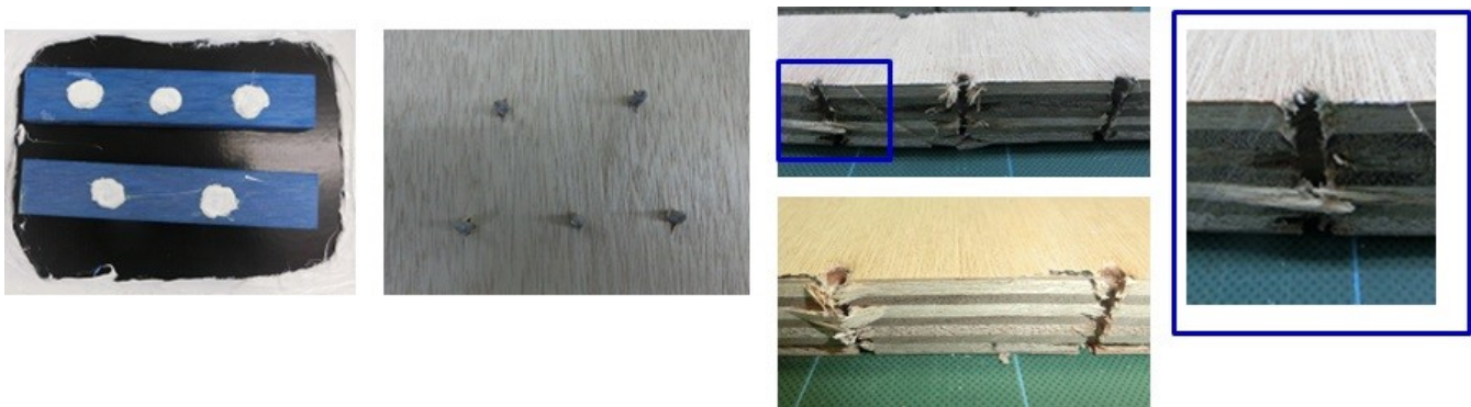
Fig.2 Appearance after specially shaped screw water seal test when we placed 3040BK
